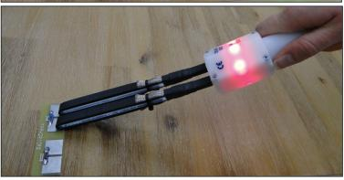
If you touch Galvocheck "bad", the red LED shall light up and an acoustic signal sounds. If not, do not use the Galvotest, but replace the conductive coating on the test fork.
