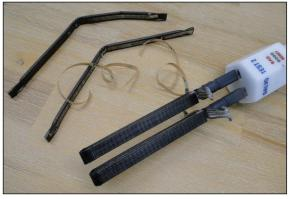
3. Secure the new conductive coating and the copper mesh with a cable tie and cut it off flush.
