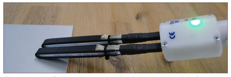
Press the test fork against an anodized object with a little force, until the green LED "good" lights up.
