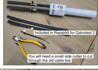
Remove the old cable ties and the worn out conductive coating by cutting the tyraps and remove the old conductive coating carefully from the testfork.
