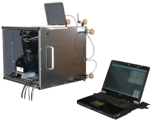
Figure 9: Mobile type A. It can be fixed onto the testing object, e.g. aircraft surface, by vacuum.
