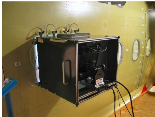
Figure 9: Mobile type A. It can be fixed onto the testing object, e.g. aircraft surface, by vacuum.
