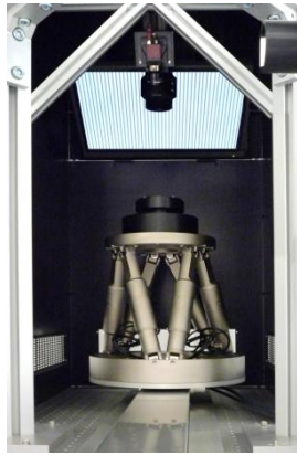
Figure 8: Desk-top type C. It is mounted in a clean room for X-ray telescope mirror manufacture.
