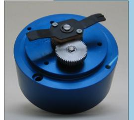
Technical data position sensor S2: Supply voltage: 2-wire, 24V DC nom. Output: 4...20mA, Shunt < 500  $\Omega$ /2...10V Range: Fullscale appr. 40° to 120° Direction: Changeable by bridge contactor Technical data gearbox: Diameter: 90mm Flange mounting: 70mm Height: 32mm Speed redution: 4:1; 10:1; opt. other Inside: Wheel set
