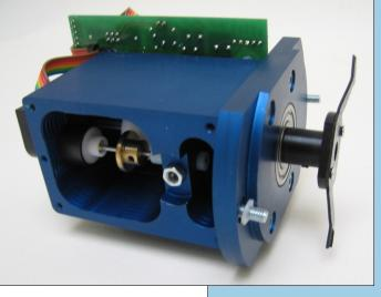
The LVDT is a high-resolution differential transformer, which generates an analogue signal in proportion to the linear movement.
